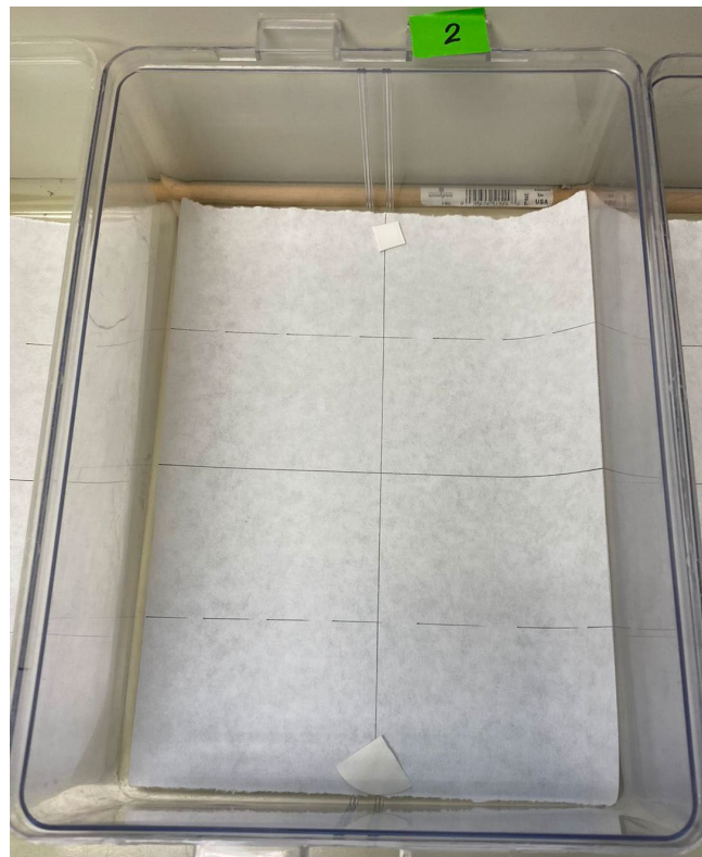
Figure 11. Plastic arena used to test attraction to commercially available lures of boll and pepper weevil. Adult males were released in the center of the arena and were free to choose between the lure or the blank filter paper (control).
