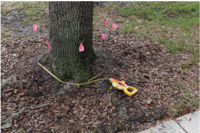
Figure 1. Image of the field method for measuring the circumference of the trunk flare. The same person took this measurement each time to ensure precision.
